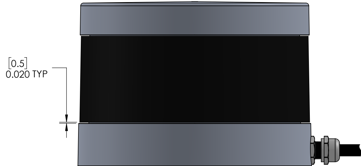
WINDOW INSTALLED MIDWAY BETWEEN LID AND SPINDLE
