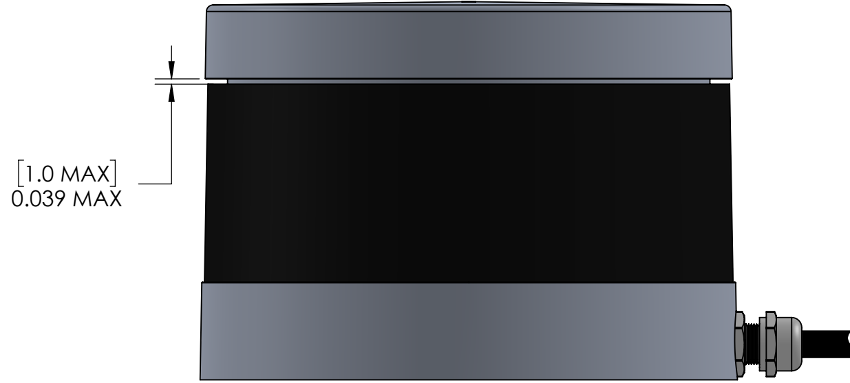
WINDOW INSTALLED FLUSH WITH SPINDLE
